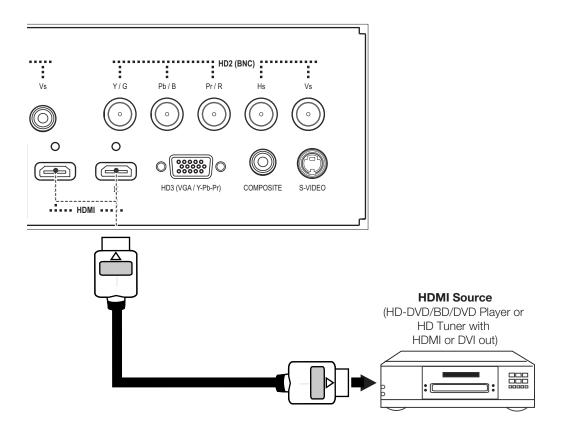
Figure 3-11. HDMI Source Connections
